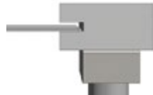
Fig. 2 Rail plate with guide rail attached
